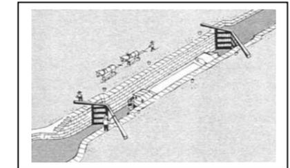
Water is let into the lock chamber from the upper elevation. Since the lower lock gates are closed, the incoming water cannot escape from the lock chamber. The
